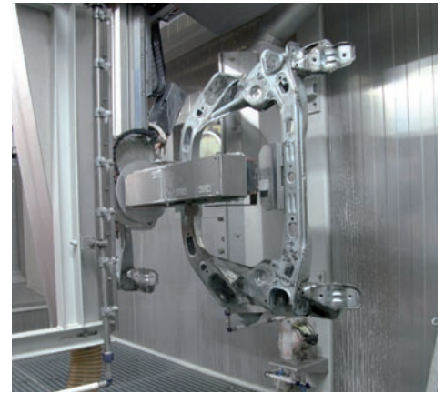
Automatic subframe drying and subsequent inhibitor processing
