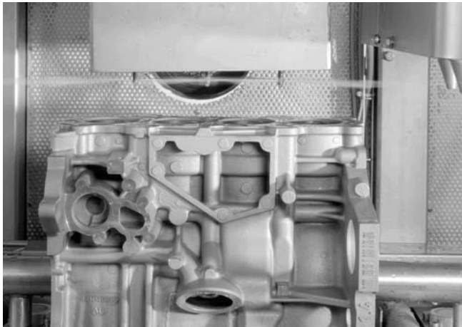
Fig. 2: Engine block in the blasting cabin for decoring with the help of high-pressure water
