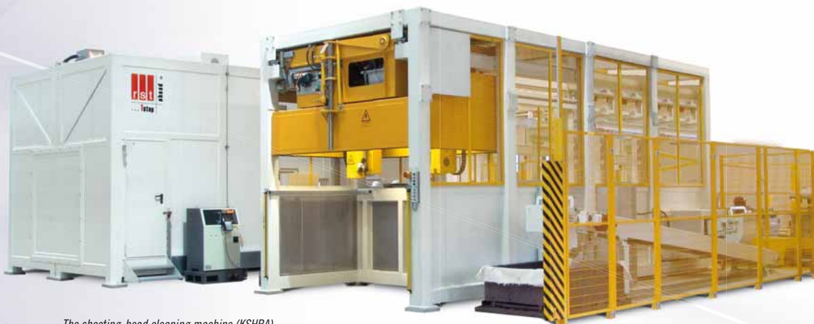
The shooting-head cleaning machine (KSHRA) by RST (foreground) as an addition to the KKRA (background). Site: Dillingen, Germany
