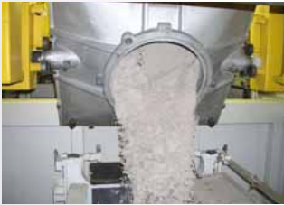
The manipulator attachment turns the head over and tips out loose sand
