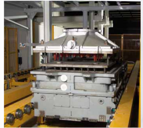
The cleaned and dried core box on its way back to the core shooter.
