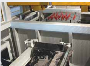
Integrated vibrating function (front), shooting head on its way to the cleaning machine (rear)
