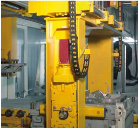
The manipulator attachments transfer the drag (foreground) and cope (left) to the cleaning operation in a fully automatic process.
