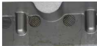
Contaminated and cleaned slotted nozzles
