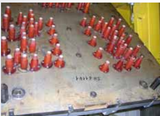
Shooter nozzles clogged with sand before cleaning
