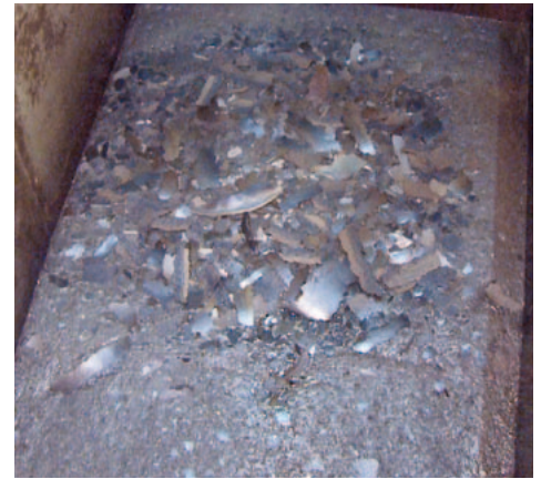
Slag residues removed from the crucible in the collection pan in the housing
