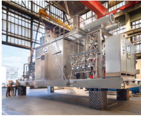
Gas turbine skid, assembled and wired ready for operation, is prepared for transport
