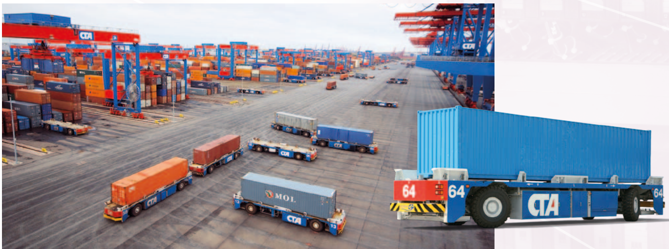
Fully automated operation with control engineering from RST: automated guided vehicles. These driverless container transfer vehicles, equipped with diesel hydraulic or diesel electric drives (AGVs and E-AGVs respectively) are responsible for the automated transfer of 20', 40' and 45' containers in the terminal. Another ideal combination of RST control engineering and RST sheet metalworking.
