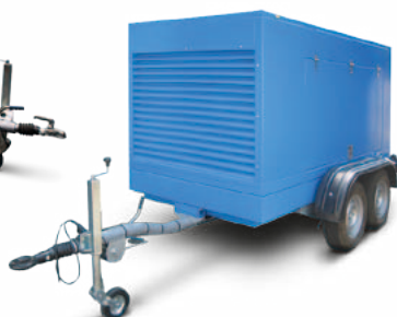
Sound insulating covers made of aluminium surrounding the motor and pump
